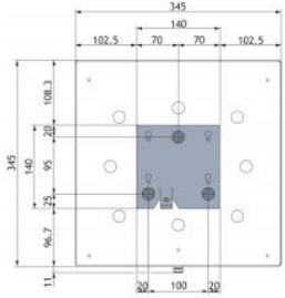
MOUNTING DETAILS BACK CONNECTOR VERSION\_x000d\_(wall mounting bracket included)
