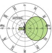
This curve shows the radiation patterns in the horizontal plane (horizontal coverage).
