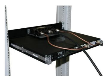
TX AND RX CABLES CAN BE SWITCHED TO HIGH OR LOW ON THE FILTER
