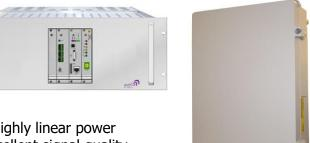
The D-CSF 3604 is a fibre optic fed TETRA repeater. The repeater is part of a system that is fed from an Axell Wireless Optical Master Unit (OMU). RF signals are coupled off from a nearby base station by the OMU, which modulates the RF to optical signals that are distributed via fibre optic cables to one or several remote D-CSF repeaters. The maximum optical loss allowed for is 10 dB of fibre between the OMU and the most distant last remote unit that the OMU supports.
