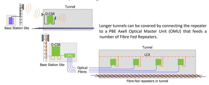
$\hbox{D-CSR 3604: 390 MHz to 395 MHz Digital channel and band selective repeater for public safety-EMEA \& APAC}\\$
