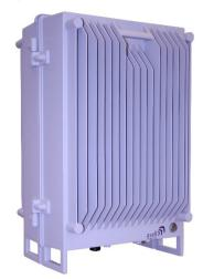
The BSF 3604 is a fibre optic fed TETRA repeater. This dual band, version processes two different (non-adjacent) bands in one enclosure. The repeater is part of a system that is fed from an Optical Master Units (OMU). The maximum optical loss allowed for is 10 dBo between the OMU and the most distant last remote unit that the OMU supports. This offers great flexibility when providing RF coverage in areas where it is not possible to rely on off air transmission.
