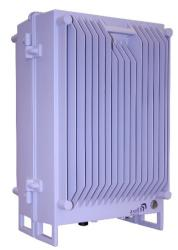
The BSF 3604 is a fibre optic fed TETRA repeater. This dual band, version processes two different (non-adjacent) bands in one enclosure. The repeater is part of a system that is fed from an Optical Master Units (OMU). The maximum optical loss allowed for is 10 dBo between the OMU and the most distant last remote unit that the OMU supports. This offers great flexibility when providing RF coverage in areas where it is not possible to rely on off air transmission.
