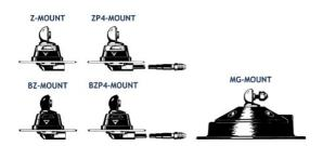
Whips from the Z/ZP4 mounts and the MG-mount are **NOT** compatible.
