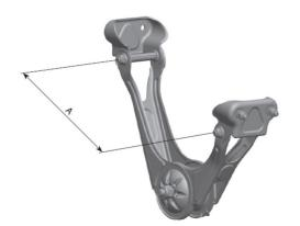
Distance "A" between the jointbolts of the downtilt kit in mm (max. 395 mm).
