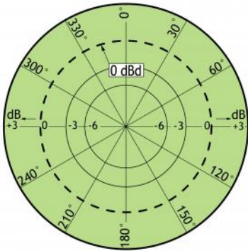
TYPICAL RADIATION PATTERN (H-PLANE)
